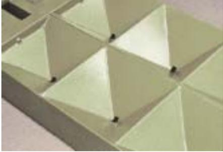
Our standard sweep-in M-Section® pneumatic recovery systems efficiently recover and recycle most medium and low-density blast media, such as glass bead, plastic, and aluminum oxide. The recovery section can be placed in a shallow channel, just 10 inches deep, for a true sweep-in operation, or surface mounted where conditions will not allow excavation.
